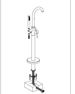
Please check that your pressure is suitable for this product before installation, details can be found on our website, recommed minimum working pressure: 0.5 bar, maximum working pressure: 3 bar
